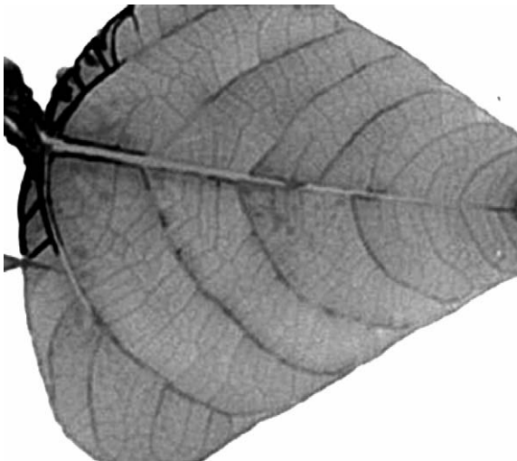
Fig. 6. Neutron-induced electron radiography of a plant showing some nutrients inside the central stem.
