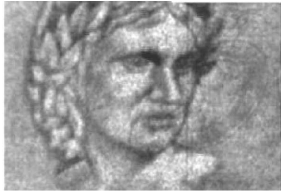
Fig. 7. Neutron-induced electron radiography of a regular Brazilian bill showing one of the security marks.
