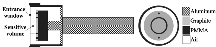
Fig. 2. Extrapolation chamber simulated using the MCNP-4C code.
