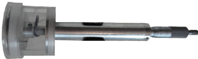
Fig. 1. Extrapolation chamber developed at IPEN (Dias and Caldas, 1998).
