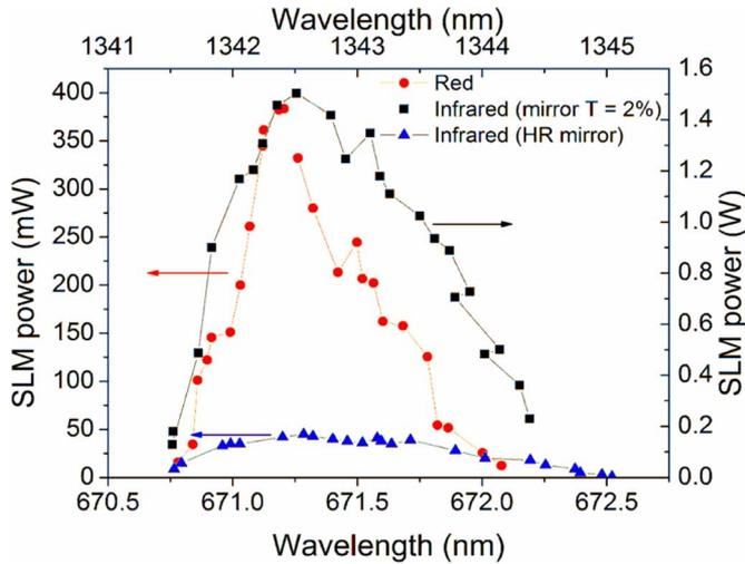
Fig. 6. Tuning curve of the red emission (circles), infrared emission when an output coupler with 2% transmission was used (squares) and infrared emission when HR mirrors were used (triangles).
