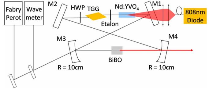
Fig. 1. Experimental setup used for an intracavity second harmonic generation of a Nd:YVO<sub>4</sub> laser.
