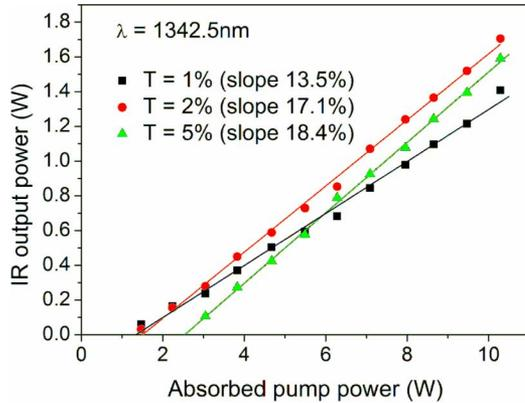
Fig. 2. Infrared output power versus absorbed pump power for different output couplers transmittance (M3), without any intracavity etalon.
