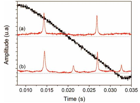
Fig. 3. Scanning confocal Fabry-Pérot spectra of the IR emission, showing SLM lasing (a) with the 40% coated thin etalon and (b) without any intracavity etalon. The scanning ramp voltage is also shown.
