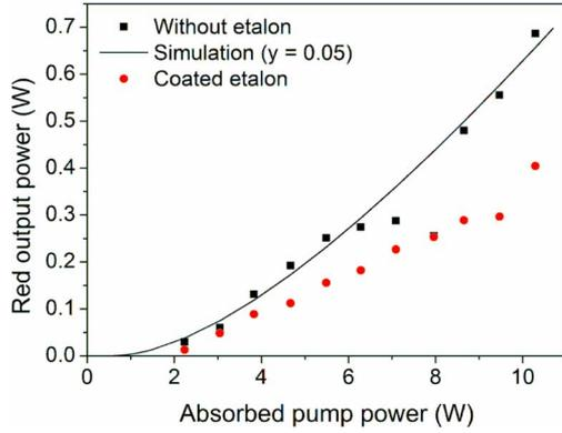
Fig. 5. Red output power versus absorbed pump power with (circles) and without (square) the  $R = 40\%$  coated thin etalon. The solid line is a fit to the theoretical formula, (2).
