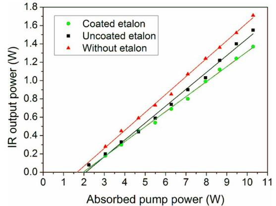
Fig. 4. FH power at 1342.3 nm versus absorbed pump power for  $T = 2\%$  output coupler transmittance. The plots with etalon relate to single-frequency power.
