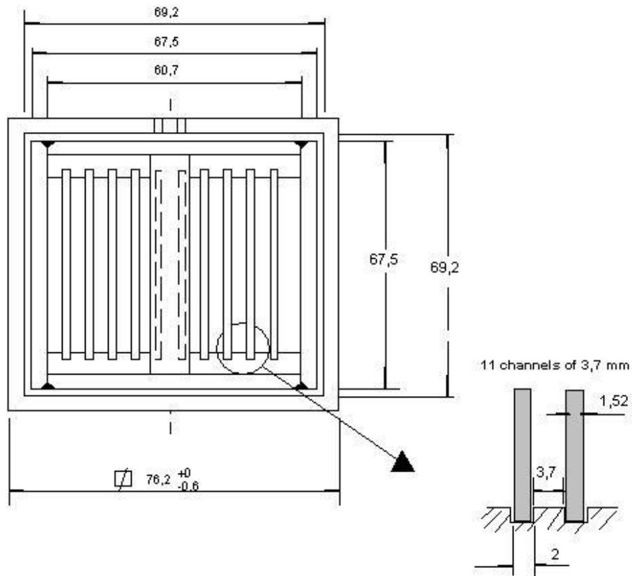
Fig 3: Cross section of the MID (dimensions in mm).
