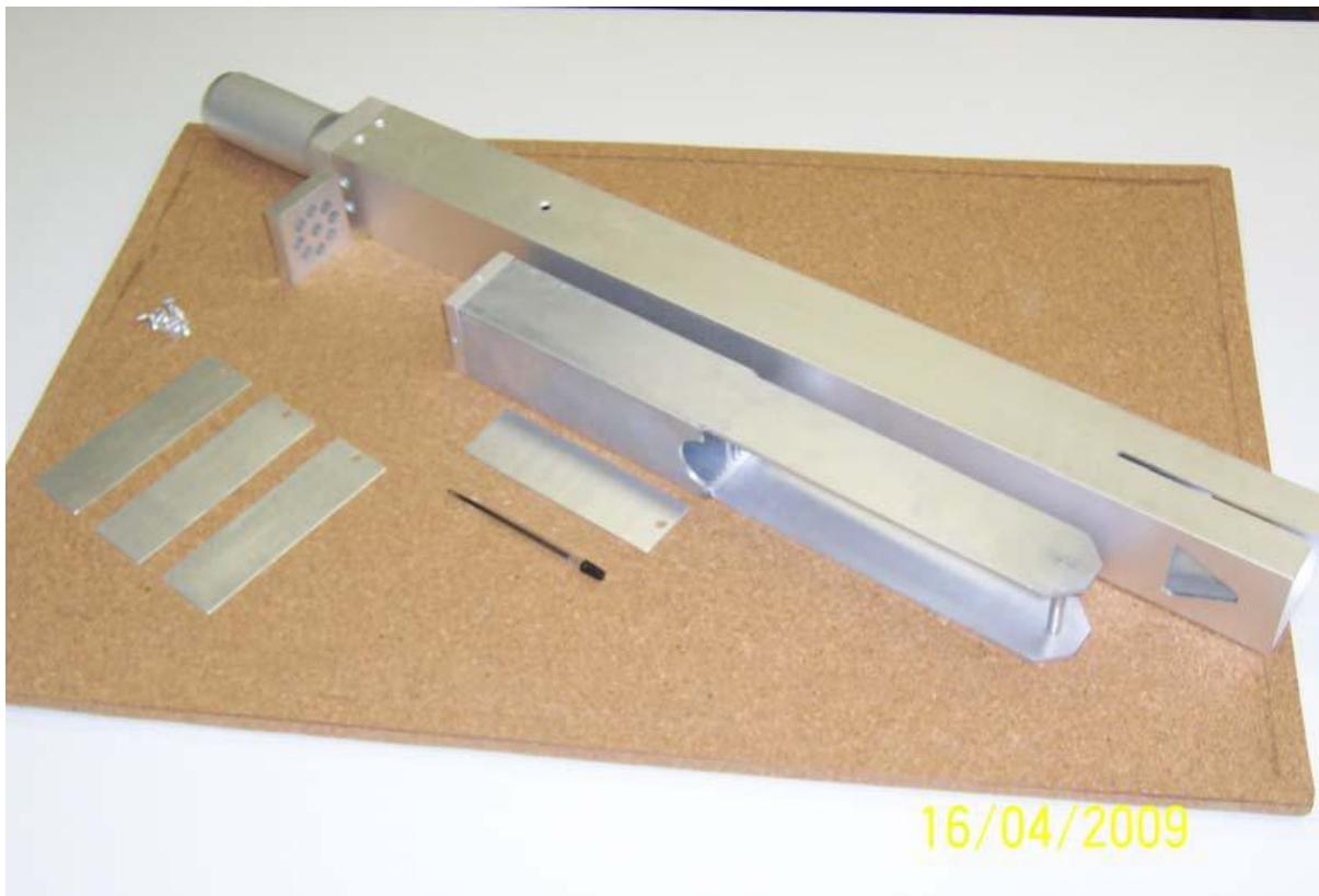
Fig 2: Miniplate irradiation device – MID.
