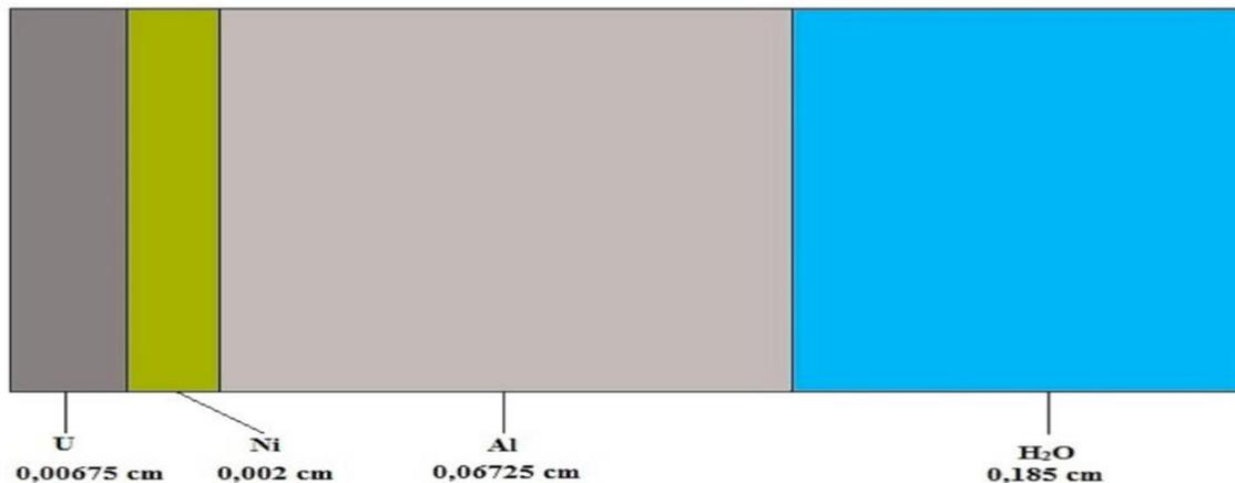
Fig 7: Half the thickness of U-Ni LEU target with plate geometry (67.5  $\mu\text{m}$ ), nickel foil, aluminum plate and cooling channel.
