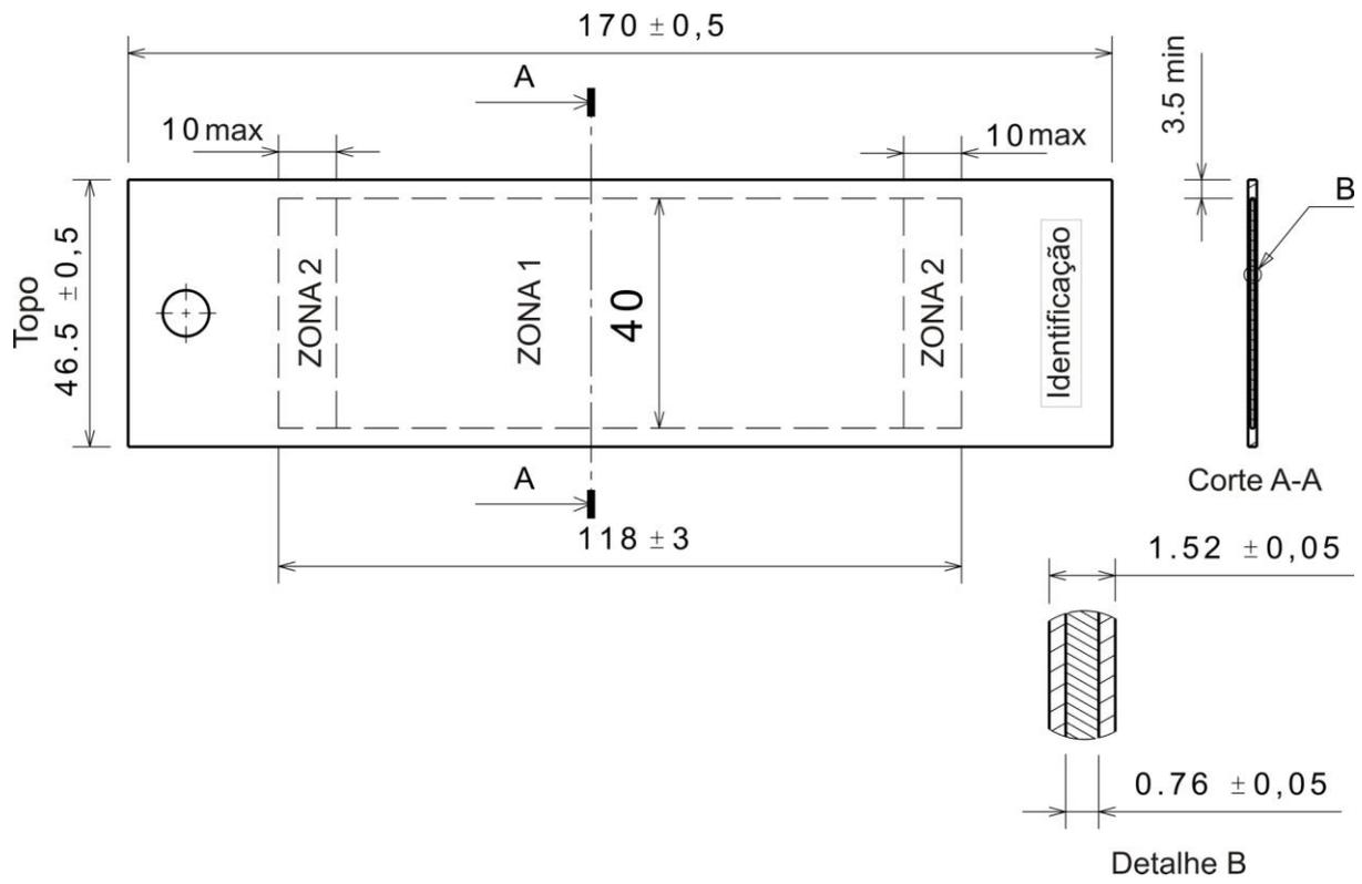
Fig 1: UAix-Al miniplate dimensions.
